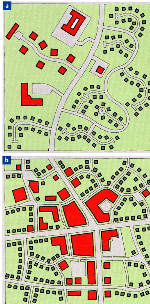
(a) dispersed and car-dependent versus (b) compact and walkable layout Source: DfT (2007) Manual for Streets (ref. 4)
